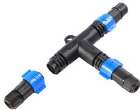
9. IP67 Water Tight Connecting Device with Distribution block, 3 pole, 1 input, 2 outputs, Cable Diameter 4.5 - 11mm. [DMX] Ordering Code: AUN-CON-0023-00
