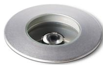
The POLKA family of projectors and ground-recessed luminaires is characterized by a small size. The forged aluminum housing exhibits exceptional strength against mechanical impact and corrosion resistance. Several light distributions and color temperatures are available as a standard option. POLKA is equipped with the UniBlock anti-humidity kit for improved reliability and resilience against ingress of moisture. POLKA is also available in stainless steel, refer to the ATOM family for details.
