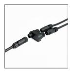
Ordering Code: AUN-CON-O012-OO IP68 connection device 5 pole, cable diameter 7.1-13mm, with distribution block , 1-10V or DALI
