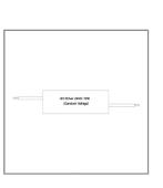
Ordering Code: AUN-DRG-0027-00 LED constant voltage driver, 24VDC, 72W
