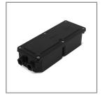
Ordering Code: AUN-DRG-0021-00 LED constant current driver, 1050mA, 38W, with IP67 GFR polymer enclosure. 1-10V
