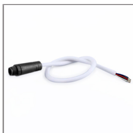
Ordering Code: ATR-CON-0002-00 Feed in cable 5x0.75sqmm, L= 2000mm, for RGBW luminaire, with M12 connector
