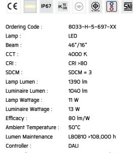
Input Voltage: 220-240Vac 50/60Hz
