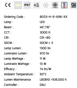
Input Voltage: 220-240Vac 50/60Hz
