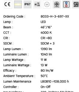
Input Voltage: 220–240Vac 50/60Hz
