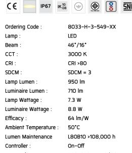
Input Voltage: 220-240Vac 50/60Hz
