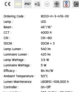
Input Voltage: 220–240Vac 50/60Hz
