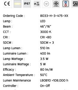
Input Voltage: 220–240Vac 50/60Hz
