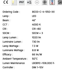
Input Voltage: 220–240Vac 50/60Hz
