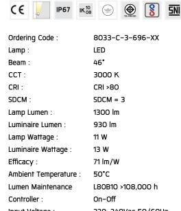
Input Voltage: 220–240Vac 50/60Hz
