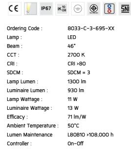
Input Voltage: 220-240Vac 50/60Hz
