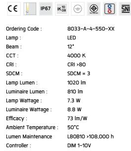
Input Voltage: 220–240Vac 50/60Hz
