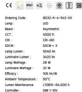
Input Voltage: 220-240Vac 50/60Hz
