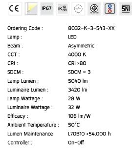
Input Voltage: 220–240Vac 50/60Hz
