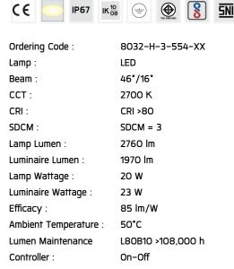
Input Voltage: 220-240Vac 50/60Hz
