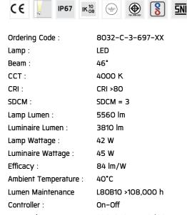
Input Voltage: 220-240Vac 50/60Hz
