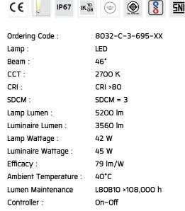
Input Voltage: 220-240Vac 50/60Hz
