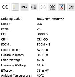
L80B10 >108,000 h DIM 1-10V 220-240Vac 50/60Hz 4.60 kg.
