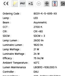
Input Voltage: 220-240Vac 50/60Hz
