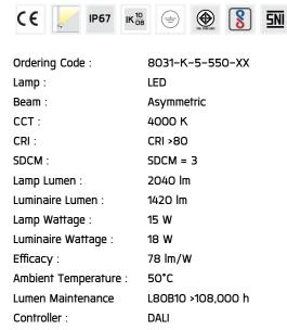
Input Voltage: 220-240Vac 50/60Hz
