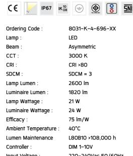
Input Voltage: 220-240Vac 50/60Hz
