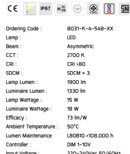
Input Voltage: 220-240Vac 50/60Hz
