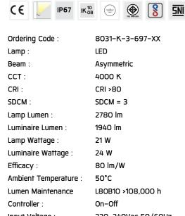
Input Voltage: 220-240Vac 50/60Hz
