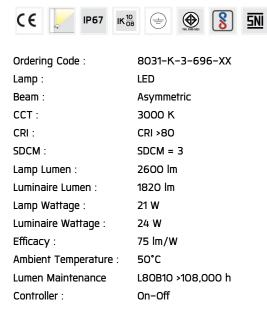
Input Voltage: 220-240Vac 50/60Hz
