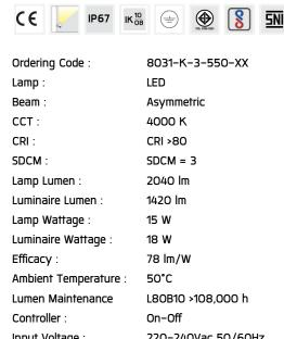
Input Voltage: 220-240Vac 50/60Hz
