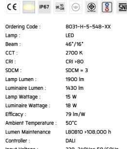
Input Voltage: 220-240Vac 50/60Hz
