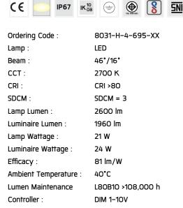
Input Voltage: 220-240Vac 50/60Hz
