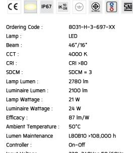
Input Voltage: 220–240Vac 50/60Hz
