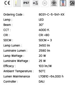
Input Voltage: 220-240Vac 50/60Hz
