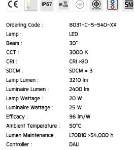
Input Voltage: 220–240Vac 50/60Hz
