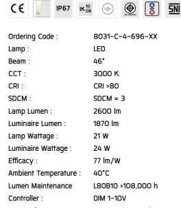
Input Voltage: 220-240Vac 50/60Hz
