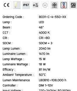
Input Voltage: 220-240Vac 50/60Hz
