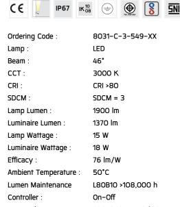
Input Voltage: 220-240Vac 50/60Hz
