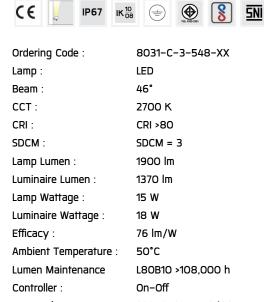
Input Voltage: 220-240Vac 50/60Hz
