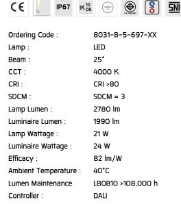
Input Voltage: 220-240Vac 50/60Hz
