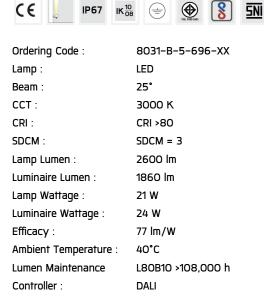
Input Voltage: 220-240Vac 50/60Hz
