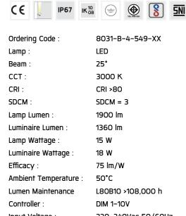
Input Voltage: 220-240Vac 50/60Hz
