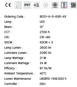
Input Voltage: 220-240Vac 50/60Hz
