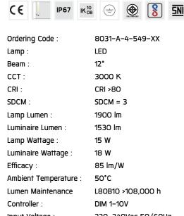
Input Voltage: 220–240Vac 50/60Hz
