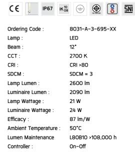
Input Voltage: 220-240Vac 50/60Hz
