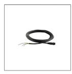
Ordering Code: ATR-CAB-0004-00 Feed in cable L = 1000mm 2x1sqmm + 3x0.5sqmm suitable for RGBW luminaire.
