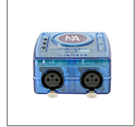
Ordering Code: AUN-DMX-0025-00 DMX controller, 2-Channel
