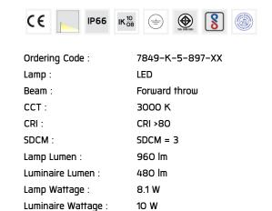
Ambient Temperature : 50°C Lumen Maintenance L70B10 >66,000 h
