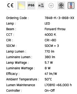
Input Voltage: 220–240Vac 50/60Hz
