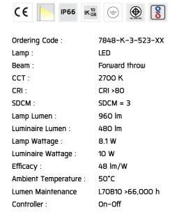
Input Voltage: 220–240Vac 50/60Hz
