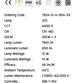
Input Voltage : 220–240Vac 50/60Hz
