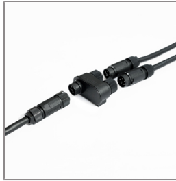
Ordering Code: AUN-CON-0012-00 IP68 Water Tight Connecting Device with Distribution block, 5 pole, 1 input, 2 outputs, Cable Diameter 7.1 – 13mm. [1-10V or Dali]
